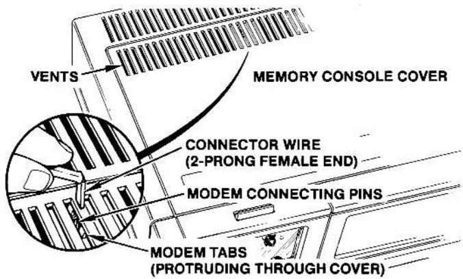
**Step 5.** Look at the two modem tabs protruding through the vent hole on the Memory Console. Take the two-prong connector end of the connector wire and push it through the vent hole until it plugs into the two pins on the top side of the modem. If you can still see either of these pins after you've plugged in the two-prong connector, then you haven't made a proper connection. Re-align the two-prong connector with the modem pins and plug it in again.
