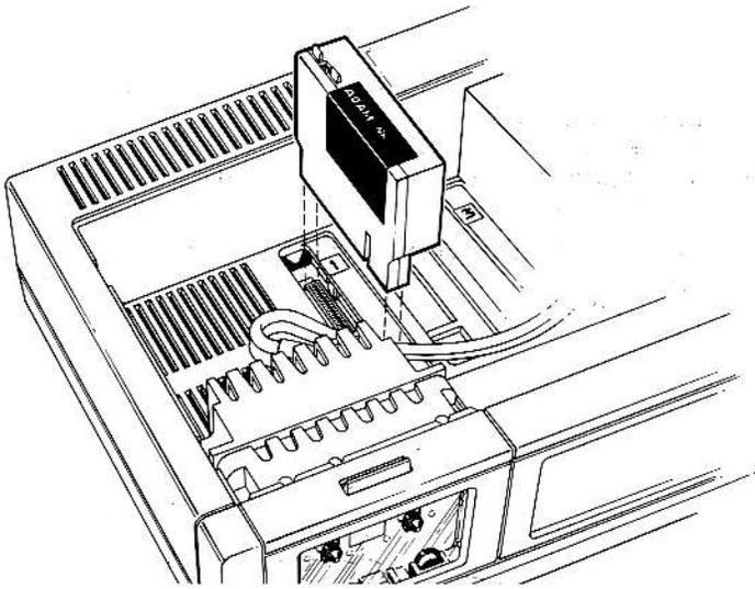
**Step 2.** Look inside the Memory Console. There are three expansion ports. These expansion ports are labeled 1, 2, and 3 on the plastic casing to their right.
